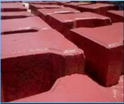
Bricks made from sludge, a by-product of the effluent treatment system.
