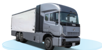
Prima H.28 Indigenously developed H2 ICE truck with a range of ~550km
