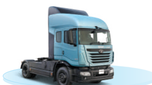
Prima E.55S Battery electric prime mover to decarbonise logistics operations across sectors
